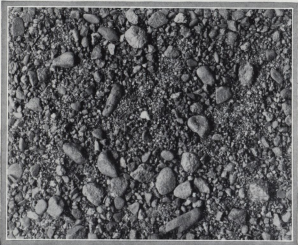
Medium Sand, an Actual Sample, Full Size
