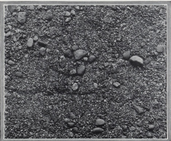
Fine Sand, an Actual Sample, Full Size
