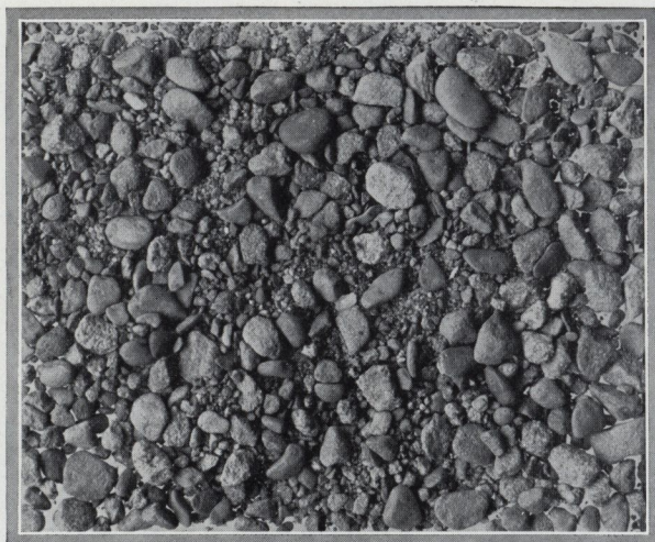
Coarse Sand, an Actual Sample, Full Size
